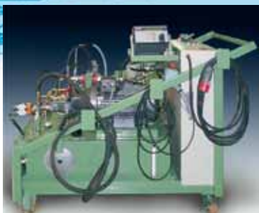
FUM Flushing Unit: Flushes the system to a specific cleanliness before commissioning.
