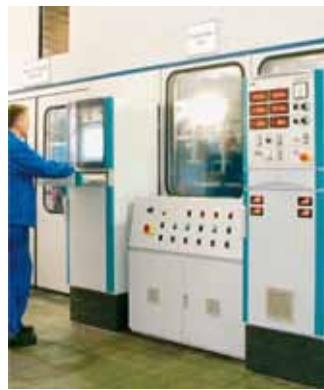
Lubrication oil supply for wind turbine transmission test rig.
