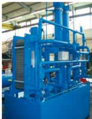
Lubrication oil supply for wind turbine transmission test rig.
