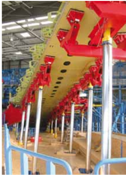
Total-cell fatigue test system for the Test Airbus A 380.
