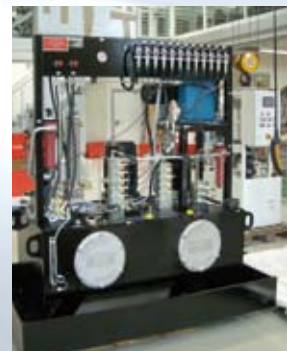
Power units for pressure supply to clutch / brake, cooling, lubrication and additional functions
