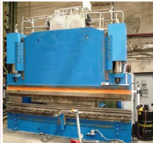
Modernisation of press brake: New hydraulics incl. pipework, new electric control panel. Cylinder synchronization: \pm 0.01\text{ mm/1m} , on-site commissioning
