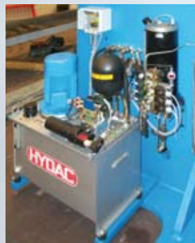
Power units for pressure supply to clutch / brake, cooling, lubrication and additional functions
