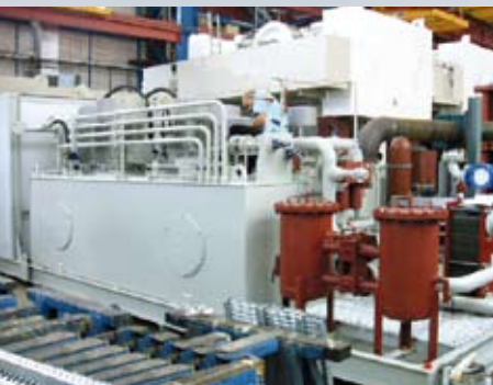
Large power unit, V = 7000 \text{ l}
