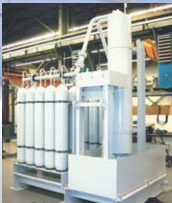
Standard piston accumulator station for the automotive industry
