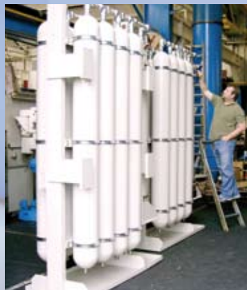
Bladder accumulator station for IHU presses
