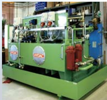
Power units for pressure supply to clutch / brake, cooling, lubrication and additional functions
