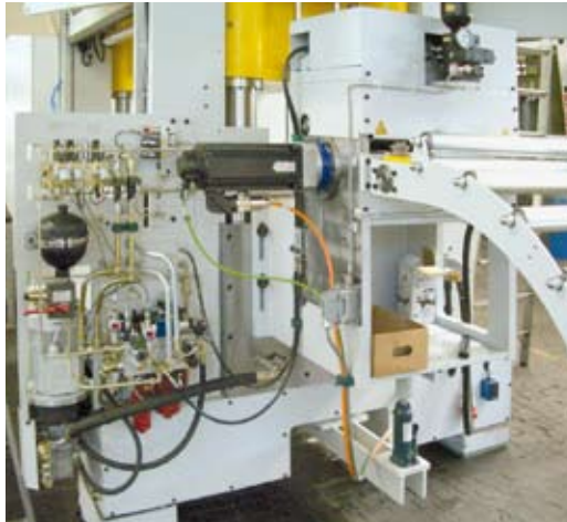
Hydraulic power unit in straightening press: 5,000 kN
